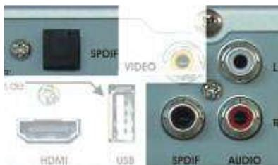
If your amplifier or Dolby-Surround-Decoder have an optical or electrical digital input, connect an appropriate SPDIF port over a suitable cable to the digital input on your amplifier or Dolby-Surround-System. You can enjoy Dolby-Digital-Surround-Sound – AC3 in your Home cinema only over these ports. But it is necessary that the chosen program supports this standard.
