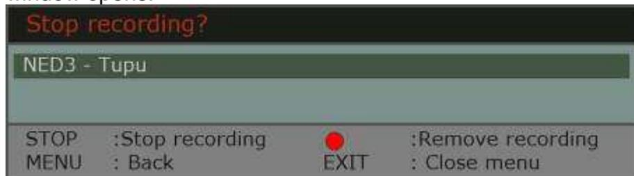
You can stop the recording now by pressing the Stop button. In this case the time shift recording will be handled as a normal recording and saved on the storage medium. If you do not want to save the recording, so press the red button to delete the recording directly.
