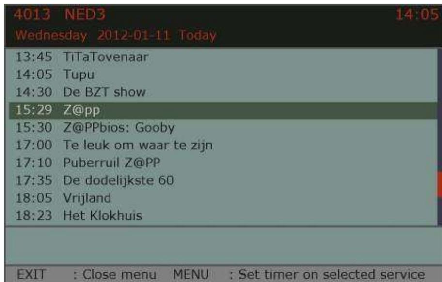
Press cursor keys to select the program that you want to record with the help of timer. If the corresponding entry is darkened, so press the „Menu“ button to use the data in the timer. Then the window opens like for the manual recording and you can edit the used data. By pressing the button „Rec“ you will use the data in the timer list. Positions that are already programmed will be shown in red.
